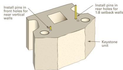
Figure 3 - Installation of Pins
