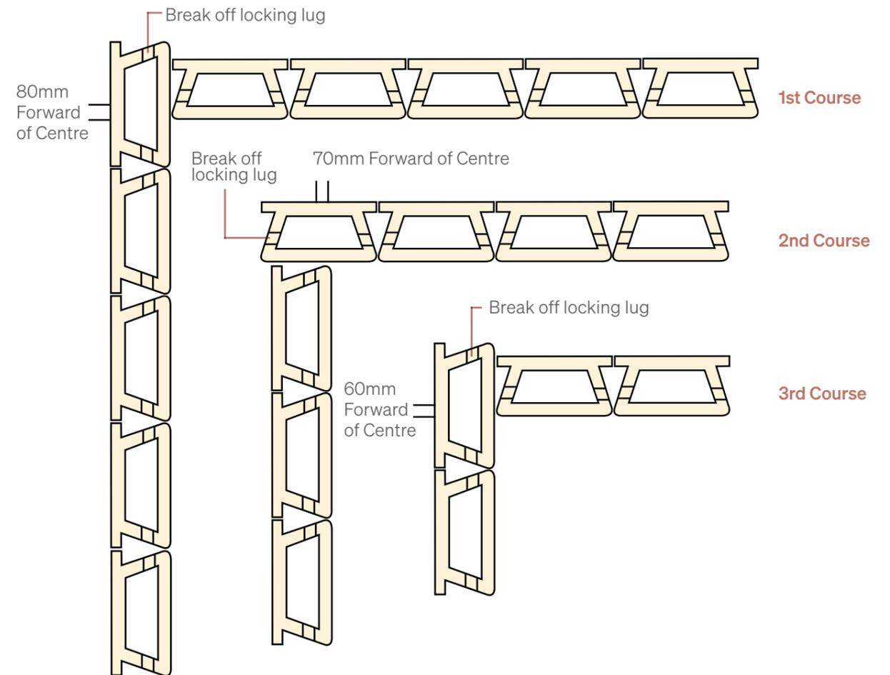
The above applies to installation of a retaining wall at 8 courses high.
