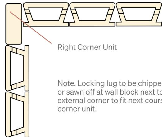
Note. Locking lug to be chipped or sawn off at wall block next to external corner to fit next course corner unit.
